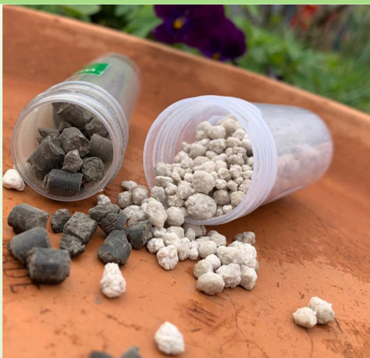
A struvite, ammonium sulphate and potassium chloride granule (white) and the same compounds pelleted with dewatered food waste sludge (left). Image by NSVA.
