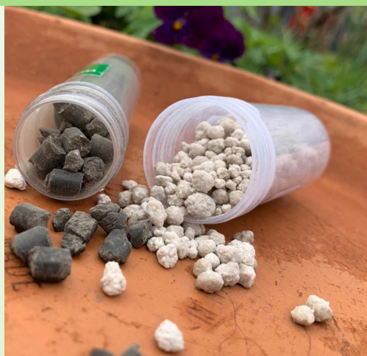
A struvite, ammonium sulphate and potassium chloride granule (white) and the same compounds pelleted with dewatered food waste sludge (right). Image by NSVA.
