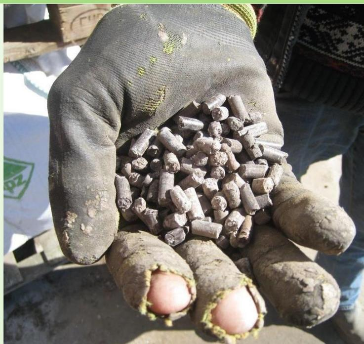
*Organo-mineral pellets from digested sludge and recovered mineral fertiliser products. Image by NSVA.*
